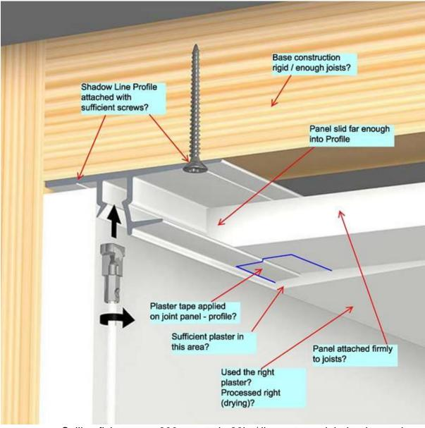
Ceiling Attached Shadowline rail 10/13mm (fix & finishing tips)
